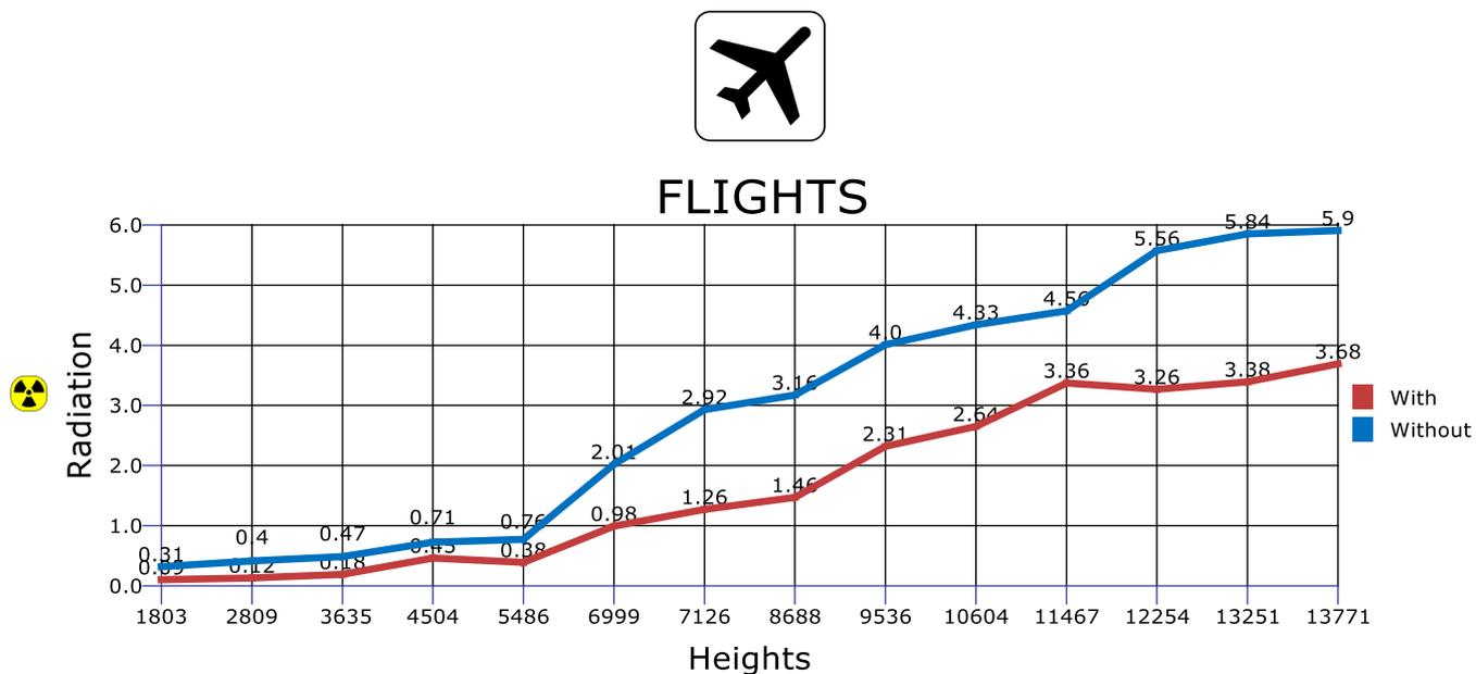
Fig 1. The measured level of radioactivity (in hundreds of micro-Roentgen) inside the plane with and without opening energy channels.
