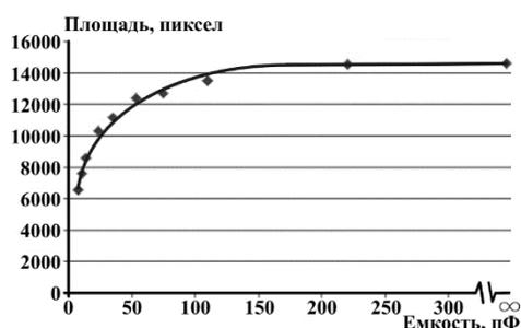
Optimal sensitivity is observed on increasing part of the curve, the choice of which is due to both the circuit elements of the device, and the parameters of the environment.
