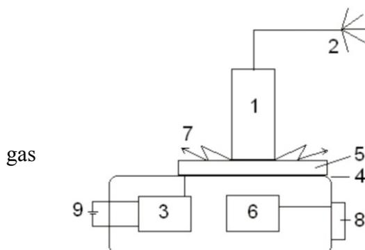
Fig. 1 The experimental setup. 1 - metal cylinder; 2 Antenna "GDV Sputnik"; 3 - high-voltage pulse generator; transparent conductive coating; 5 - transparent quartz electrode; 6 - video converter; 7 - discharge; 8 - USB-drive; 9 - Power Supply
