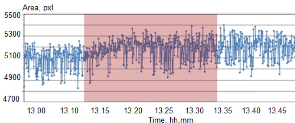
Fig. 8. Change in GDV signal during the experiment; red area allotted time of low-intensity sound 20Hz frequency operation.
