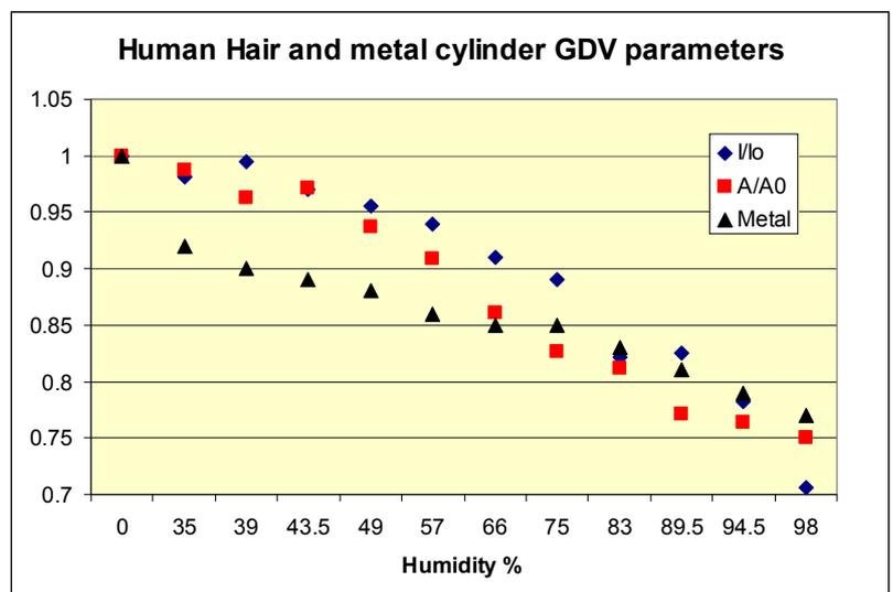
Fig. 1. Humidity dependence of Area and Intensity of gas discharge images of swatch of fresh human hair and metal cylinder expressed as a proportion – value of the parameter at 0% is the divisor.
