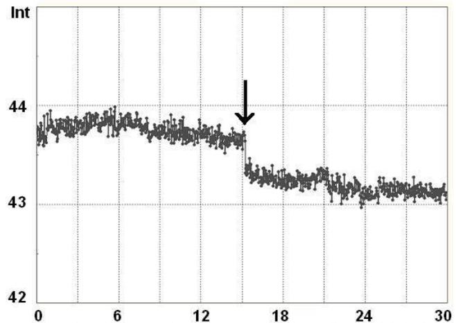
Fig. 6. Example of a 30-second reading, with hair cut from the model immediately through the reading (this moment is shown by the arrow).
