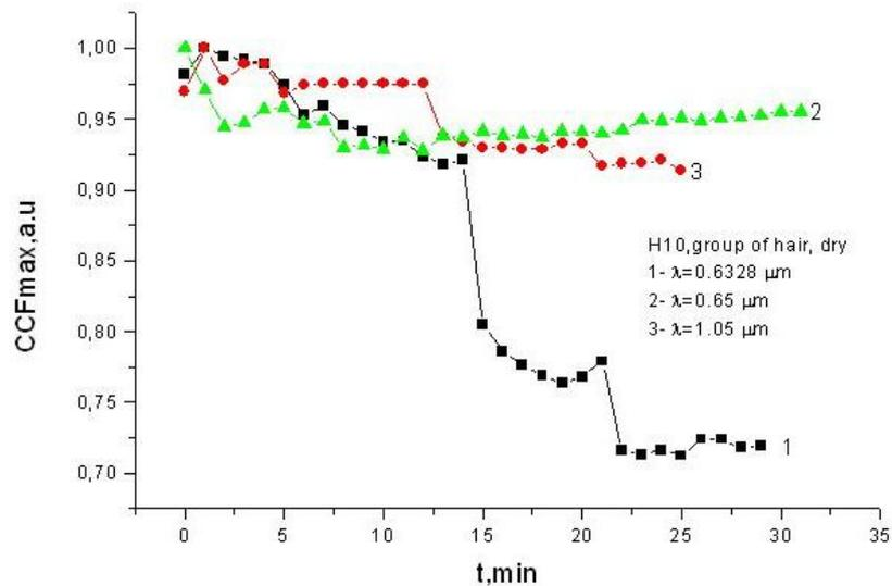
Fig.6. Mutual autocorrelation function for dry hair sample for different lasers. 1- He-Ne laser, 2- laser diode KLM-650/20, 3- infrared laser diode ESU-1005.
