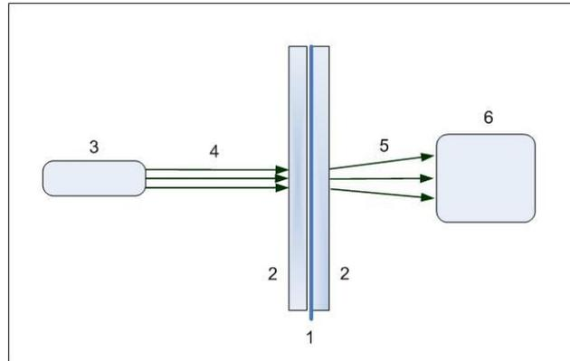
Fig.1. Laser experimental setup. 1 – single hair; 2 – optical glass; 3 – laser; 4 – coherent light; 5 – pass-through light; 6 – CCD camera.
