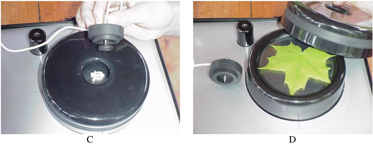
Fig.5. EPI installations for studding different subjects. A,B – low-conductive liquids; C – grains; D – leaf.
